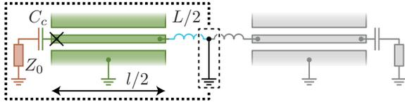
FIG. 1. Schematic diagram of the tunable resonator. For calculation of the fundamental mode frequency, the center point is connected to ground, as indicated in the dashed box. The dotted box shows the reduced circuit whose resonance frequency is to be found. The node chosen for the admittance calculation is marked by  $\times$ .
