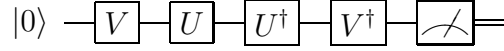
Figure 2.5: Circuit to Estimate the Average Fidelity using Random Unitaries V \in_R U(d)
