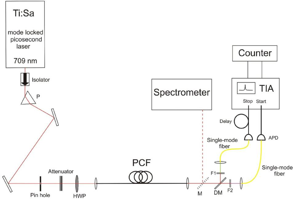
Fig. 3. Optical layout. Laser, 708 nm Ti:Sa laser; P, prism; HWP, halfwave plate; PCF, 2 m of photonic crystal fiber; M, protected silver mirror ( $R > 95\%$ ); DM, dichroic mirror (centered@700nm,  $T > 85\%$ ,  $R > 90\%$ ); F1, 570 nm band-pass filter, bandwidth 40 nm,  $T = 80\%$ ; F2, 880 nm band-pass filter, bandwidth 40 nm,  $T = 80\%$ ; APD, Silicon single photon detector.
