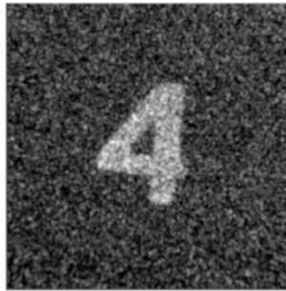
FIG. 9: Ghost image of the number 4, retrieved from the correlation function after averaging over 30000 shots.
