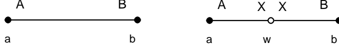
Fig. 2. Subdivision gadget. A k -local interaction is reduced to \lceil k/2 \rceil + 1 -local interactions using a mediator qubit vertex w . The operators A, B, X next to the edges indicate which operators correspond to the edges.
