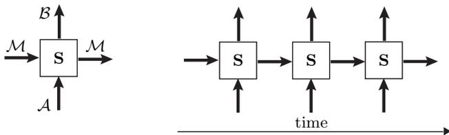
FIG. 1: *Left*: A quantum memory channel with input register  $\mathcal{A}$ , output register  $\mathcal{B}$ , and memory system  $\mathcal{M}$ . — *Right*: A threefold concatenation  $S_3$  of memory channels, with time running from left to right, and coded information running from bottom to top.
