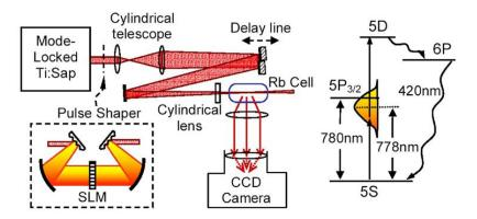
Fig. 3: Experimental configuration and relevant level diagram for atomic Rb. The cylindrical telescope weakly focuses the beam into the Rb Cell, the delay line controls the interference and the CCD records the image of the fluorescence spot. The cylindrical lens in front of the cell tightly focuses the beam in the perpendicular dimension.
