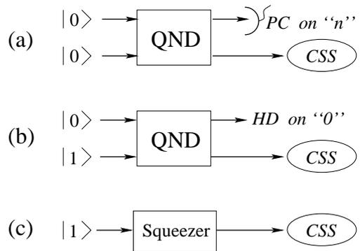
FIG. 1: A schematic of the simplification of the CSS generation. *PC* represents photon counting and *HD* represents homodyne detection. (a) Conditional production using QND with photon counting, (b) conditional production using QND with homodyne detection, and (c) deterministic production only by squeezing a single photon.
