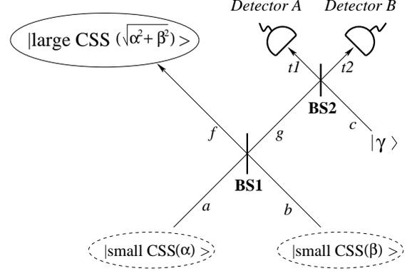
FIG. 4: A schematic of the non-deterministic CSS-amplification process. Two small CSSs at modes  $a$  and  $b$  are added to produce a larger CSS at mode  $f$  by a conditional measurement using detectors  $A$  and  $B$ . See text for details.
