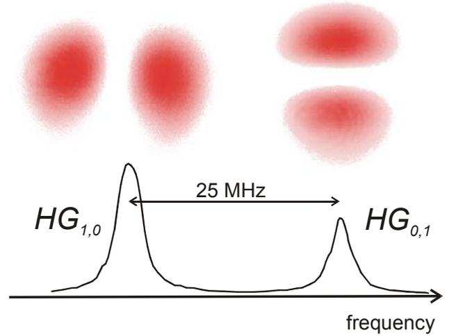
Figure 2: Higher-order modes. The measured transverse intensity distributions of the  $HG_{1,0}$  and  $HG_{0,1}$  modes is shown in the upper part. For ideal spherical mirrors, the frequencies of these modes would be degenerate. The intensity transmitted through the cavity when scanning the frequency of the excitation laser is displayed in the lower part. The experimentally observed splitting is 25 MHz.
