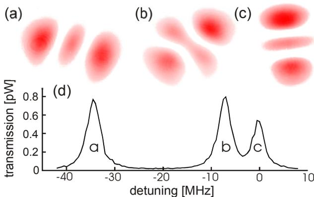
Figure 3: Higher-order modes. The spatial pattern of the three modes of order  $N=2$  are shown in (a)-(c). The resonance frequencies of the modes as determined by scanning the frequency of the excitation laser are indicated in (d).
