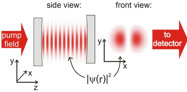
Figure 1: Sketch of the optical standing-wave cavity with a measured  $HG_{1,0}$  transverse mode depicted.
