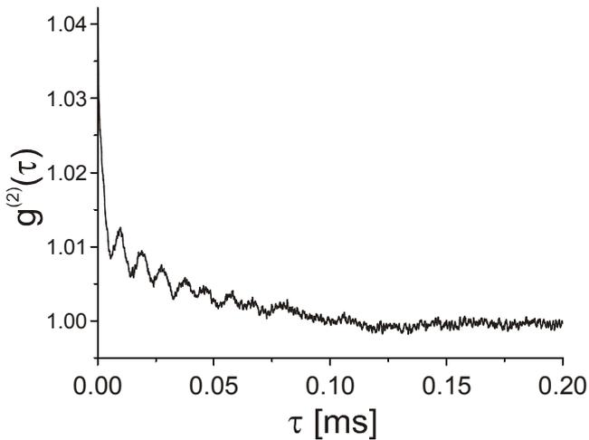
Figure 6: Autocorrelation function of single-atom transits through a  $HG_{0,10}$  mode. The detuning of the laser from the atom and the cavity are  $\Delta_A/2\pi = -50$  MHz and  $\Delta_C/2\pi = -1.5$  MHz, respectively. The motion of the atoms through many of the 11 local intensity maxima of the mode can clearly be discriminated. The function is normalised to approach 1 for large  $\tau$ .
