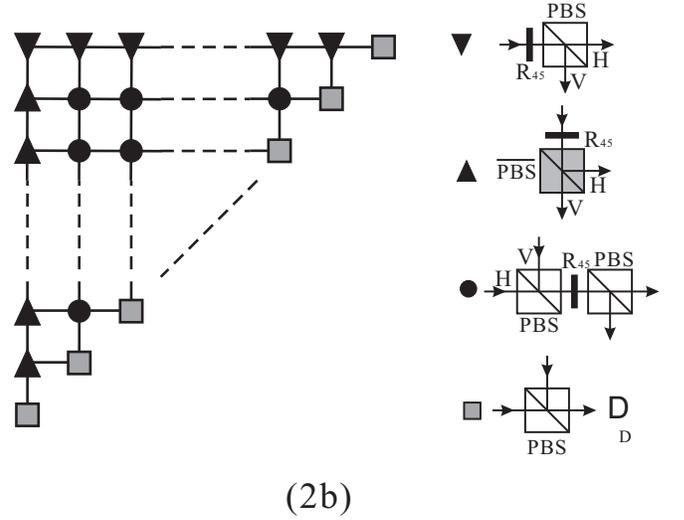
FIG. 2: Schematic of the setup to implement quantum random walk on a line with three steps (2a) and the optical network with  $N$  steps (2b).
