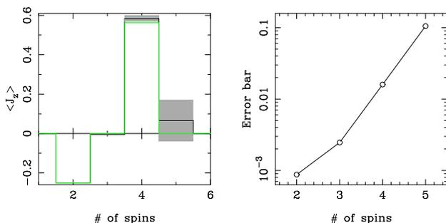
FIG. 7: Left: Plot of  $\langle S_z \rangle$  for different number of spins in a completely symmetrical state. A total of  $10^6$  measurements for each mean value was performed in this simulation. Right: Semilog plot of the error bars *vs* the number of spins. Notice the exponential increase in the statistical errors.
