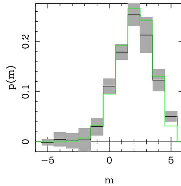
FIG. 3: Diagonal elements of the matrix given in Fig. 2. The statistical error bars are obtained by dividing the measurements into 10 statistical blocks. The solid line indicates the theoretical value.
