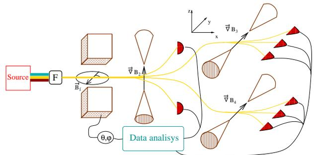
FIG. 9: Experimental apparatus for the tomographic reconstruction of the spin states of systems composed of three spin  $\frac{1}{2}$  states.
