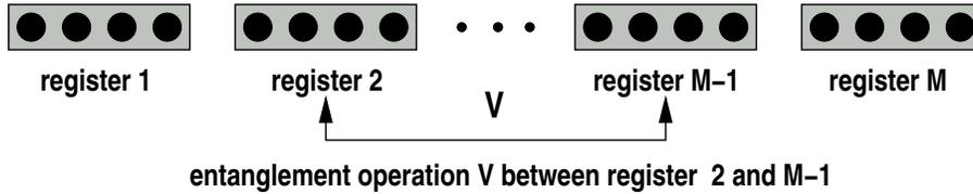
Figure 3: Schematic representation of an array of qubits consisting of  $M$  basic registers. Each basic register carries a logical qutrit of the jump code  $1 - JC(4, 2, 3)$ . Any two basic registers, such as registers 2 and  $(M - 1)$ , can be entangled by the entanglement gate  $V$ .
