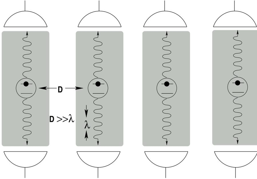
Figure 1: Schematic representation of an array of distinguishable qubits whose spontaneous emission times  $t_i$  and error positions  $\alpha_i$  are monitored continuously by photodetectors.
