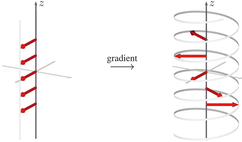
FIG. 8: Effect of a pulsed gradient field along the  $z$  axis in the rotating frame. Initial  $x$ -magnetization is assumed. A spin at  $z = 0$  is not affected, but the ones above and below are rotated by an amount proportional to  $z$ . As a result, the local planar magnetization follows a spiral curve.
