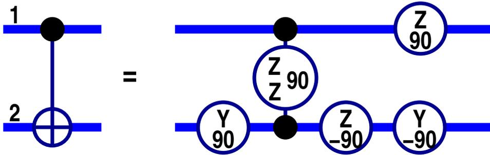
FIG. 9: Quantum network for implementing the controlled-not using operations available in NMR. The conventions for depicting gates are as explained in [2]. The two one-qubit  $z$ -rotations can be implemented by a change in the reference phase of the rotating frame without applying any RF pulses.
