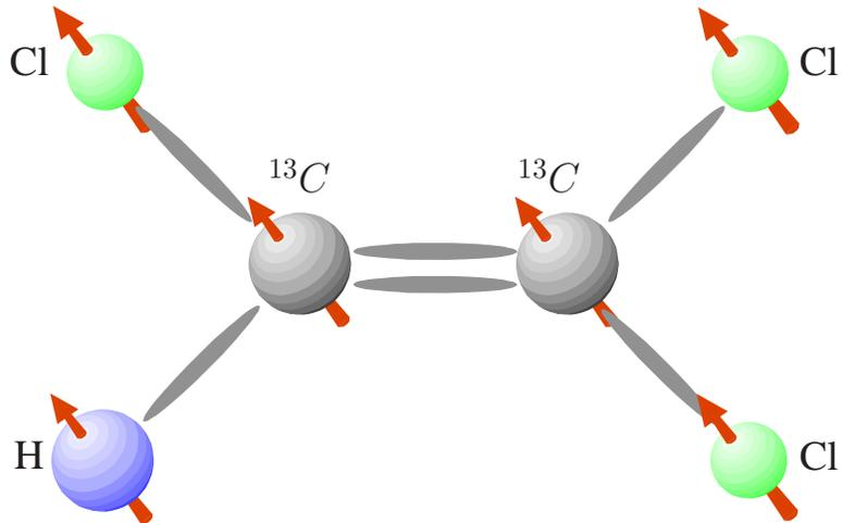
FIG. 1: Schematic of trichloroethylene, a typical molecule used for QIP. There are three useful nuclei for realizing qubits. They are the proton (H), and the two carbons ( $^{13}\text{C}$ ). The molecule is “labeled”, which means that the nuclei are carefully chosen isotopes. In this case, the normally predominant isotope of carbon,  $^{12}\text{C}$  (a spin-zero nucleus), is replaced by  $^{13}\text{C}$ , which has spin  $\frac{1}{2}$ .
