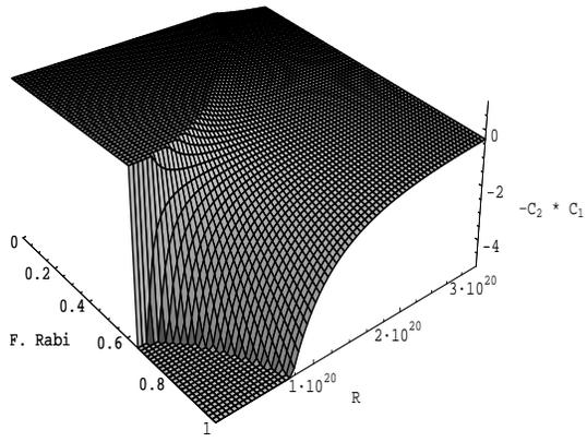
FIG. 4: The stability condition for litiio against IR Rabi frequency and pumping rate R
