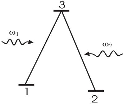
FIG. 1: The three level atom in interaction with IR Radiation.  $\omega_1, \omega_2$ , are the coupling and probe field respectively.
