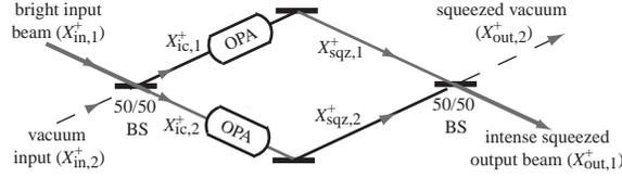
FIG. 1: Squeezed vacuum production via classical noise cancellation using two OPAs.
