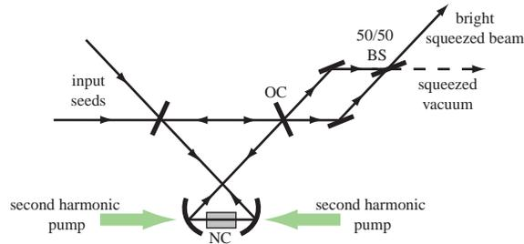
FIG. 4: Proposed scheme to cancel classical noise. OC: output coupler, BS: beam splitter, NC: non-linear crystal.
