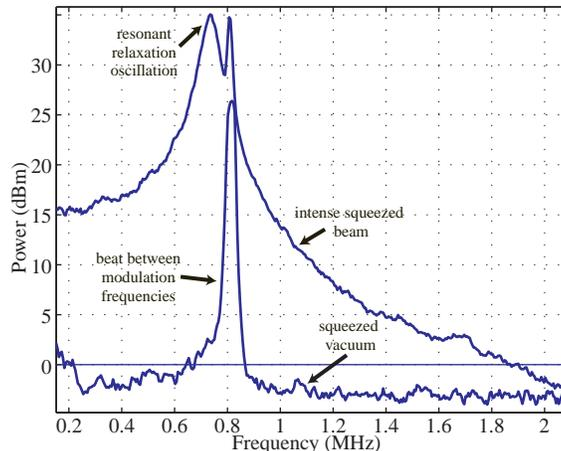
FIG. 3: Squeezing observed on the intense squeezed output (upper trace) and on the squeezed vacuum output (lower trace).
