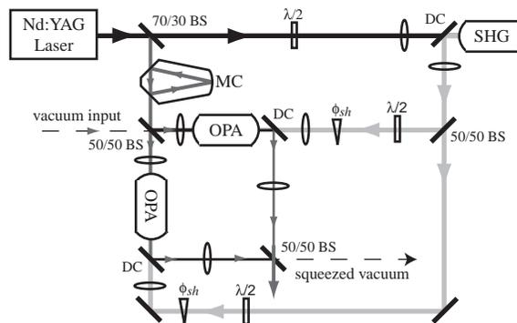
FIG. 2: Schematic diagram of the experiment. BS: beam splitter, DC: dichroic, MC: mode-cleaner,  $\lambda/2$ : half-wave plate  $\phi_{sh}$  actively controlled phase shift on second harmonic beam
