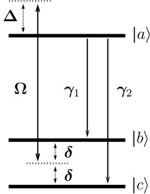
Fig. 1. The system of interest. The two lower levels  $|b\rangle$  and  $|c\rangle$  are closely spaced.
