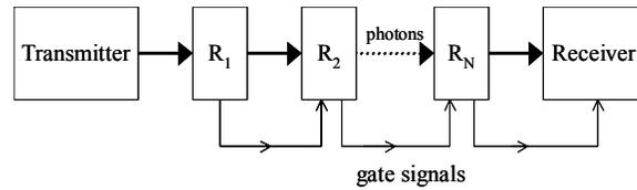
FIG. 2. A quantum relay system in which each relay  $R_i$  conditionally passes (relays) a qubit and a gate signal on to the next element provided a QND measurement indicated that a photon was actually present. The quantum relay suppresses the effects of dark counts in the receiver detectors via the gate signal, while spurious photons generated by dark counts in the relays themselves are exponentially attenuated by the transmission channel before reaching the receiver.
