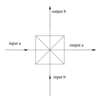
FIG. 1. A schematic diagram for the beamsplitter operation. Both the input and the output are two mode states. The different mode is distinguished by the propagating direction of the field.
