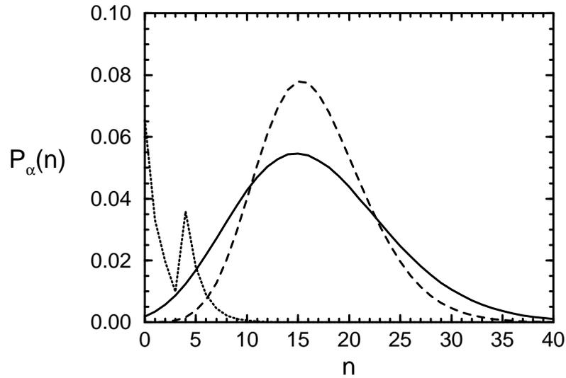
FIG. 6. The steady state distribution of photons in mode 1 (solid curve) and mode 2 (dashed curve). The parameters for the calculation are  $C_1 = C_2 = C$ ,  $n_{b_1} = n_{b_2} = n_b$ ,  $r/C = 50$ ,  $k/\kappa = 0.01$ ,  $g_2/g_1 = 2$ ,  $\kappa L = 40000\pi/\sqrt[4]{4}$  and  $n_b = 1$ . The dotted curve represents the photon distribution in mode 1 for the two-level problem when  $g_2 = 0$ . Actual values of the dotted curve are 5 times those shown.
