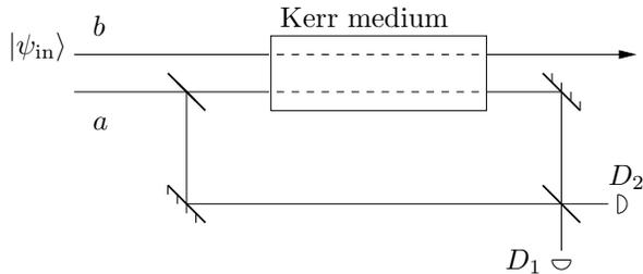
FIG. 1. A photon-number quantum nondemolition device based on the Kerr effect. A photon in mode  $b$  changes the phase of the photon in mode  $a$ . The Mach-Zehnder interferometer is tuned in such a way that a detector click in  $D_1$  signals no photon, and a click in  $D_2$  signals one photon.
