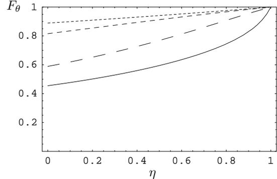
FIG. 7. The fidelity  $F_\theta$  as a function of the detector efficiency  $\eta$  for different values of  $\gamma$ . From the upper (dotted) curve to the lower (continuous) curve, the values of  $\gamma$  are 0, 0.1, 1, and 10 respectively.
