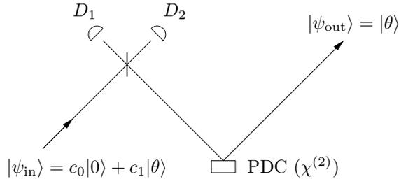
FIG. 5. Teleportation-based QND measurement device for single-photon detection that leaves the polarization of the photon intact. The device signals the presence of a single photon  $|\theta\rangle$  in the input mode with (three-dimensional) polarization angle  $\theta$ , by giving a detector coincidence in  $D_1$  and  $D_2$ .
