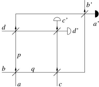
FIG. 3. Interferometric QND measurement device for single-photon detection. The device signals the presence of a single photon in mode  $a$  by giving a detector coincidence in modes  $c'$  and  $d'$  and *no* count in mode  $a'$ . The outgoing mode  $b'$  then is in a single-photon state.
