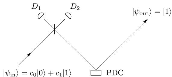
FIG. 2. Teleportation-based single-photon quantum non-demolition device. A detector coincidence in  $D_1$  and  $D_2$  signals the presence of a photon in  $|\psi_{\text{in}}\rangle$  and  $|\psi_{\text{out}}\rangle$ . This scheme breaks down when there is potentially more than one photon in the input state.
