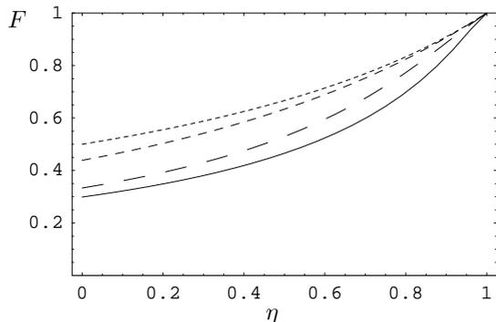
FIG. 4. The fidelity  $F$  as a function of the detector efficiency  $\eta$  for different values of  $\gamma$ . From the upper (dotted) curve to the lower (continuous) curve, the values of  $\gamma$  are 0, 0.1, 1, and 10 respectively.
