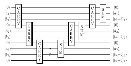
The construction of an n-bit reversible adder is a straightforward extension of the 3-bit adder. Note that an additional n qubits were needed as temporary carry bits. These qubits are reversibly set back to zero after they are used so they may be used for later computation. Therefore, even though the input and output may be stored using only 2n qubits, 3n qubits must be used for the computation.
