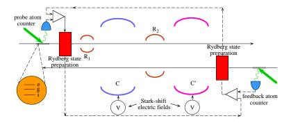
Figure 1: Schematic diagram of the autofeedback scheme proposed in this paper.  $R_1$  and  $R_2$  are the two cavities in which classical microwave pulses can be applied, C is the microwave cavity of interest and C' is the cavity automatically performing the needed correction. Electric fields can be applied at the superconducting mirrors of C and C' to Stark shift the Rydberg levels in order to tune the interaction times in C' and realize adiabatic transfer in C'
