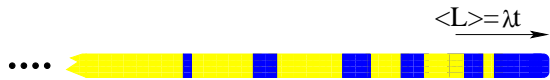
FIG. 2: (Color online) Cartoon of a microtubule in unrestricted growth. Regions of GTP + are shown dark (blue) and regions of GDP - are light (yellow). The GTP + regions get shorter further from the tip that advances as \lambda t , while the GDP - regions get longer.
