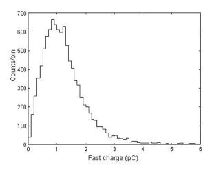
Figure 4 - Fast charge spectrum (electron component) for MIPs in chamber C (similar shapes were observed for chambers A and B), corresponding to a detection efficiency of 99 %. The counting rate during the spills was 300 Hz/cm<sup>2</sup>.
