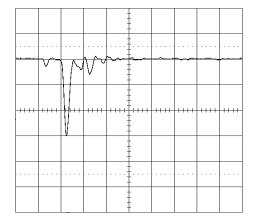
Figure 5 - Typical streamer current pulse for chamber A directly observed on a 50  $\Omega$  resistor. The horizontal scale corresponds to 20 ns/division and the vertical scale to 1 mA/division, representing each square a charge of 20 pC. A clear precursor avalanche is visible 15 ns before the main pulse which corresponds to the development and quenching of the streamer [1,2].
