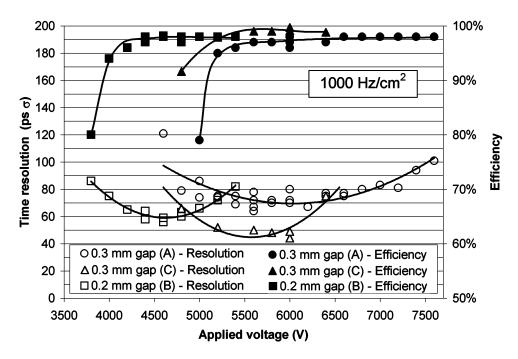
Figure 7 - Efficiency and time resolution as a function of the applied voltage. Arbitrarily shaped curves (splines) were fitted to the efficiency data and parabolic curves to the resolution data.
