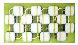
Figure 3 - Array of 16 cells mounted in a chessboard-like pattern over a printed circuit board of the ALICE-TOF project. A second layer, placed on top of this one and displaced by one pitch unit, provides a geometrical coverage better than 95%.
