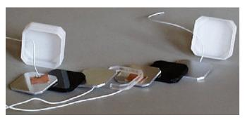
Figure 2 - Relative position of the various elements that compose one cell. The spacers (glass fibers) are the only elements not shown in the picture.
