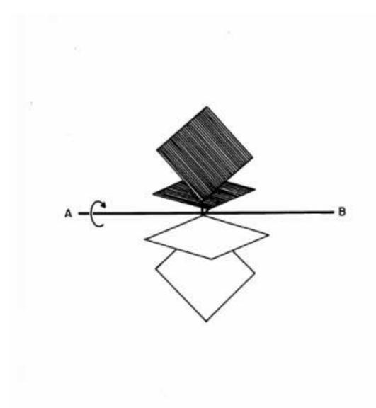
Figure 1: A variant of Crookes' radiometer is an example of chiral interaction (CI). The asymmetry in the optical absorption coefficient between the black and the silver blades generates a temperature difference between them when light is shining at the device. This expands the air close to the black blade which, in turn, pushes it around the axis AB in the preferred direction towards the black vane. This is an example of physical rather than of a geometric chirality
