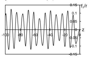
Figure 1: The gradient of dimensionless focusing field as a function of longitudinal coordinate. The bunch is d=4.7 long, and  $\alpha_0=0.2$ ,  $\delta=0.2\alpha_0$ ,  $\gamma=(1-\beta^2)^{-1/2}=10$ .
