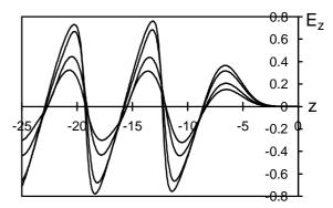
Figure 4: Accelerating electric field of two-dimensional nonlinear wake wave in nonuniform plasma with  $\sigma_p=11$  for *r*=0, 2, 4 and 5 in the order of magnitude reduction. The bunch parameters are the same as those in Fig. 2.
