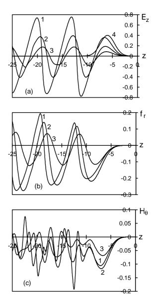
Figure 2: The two-dimensional nonlinear wake wave in uniform plasma. The parameters of the bunch are:  $\alpha_0=0.4$ ,  $\sigma_z=2$ ,  $\sigma_r=5$ ,  $\gamma=10$ . (a). The longitudinal electric field. 1-r=0; 2-r=4; 3-r=6; 4-the density of bunch at the axis  $\alpha(z, r=0)$ . The focusing field  $f_r=H_0-E_r$  (b) and magnetic field strength (c). 1-r=2; 2-r=4; 3-r=6.
