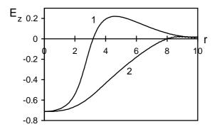
Figure 3: The radial behavior of accelerating electric field strength  $E_z$ .  $1-E_z(z=-25, r)$  in the nonlinear wake wave excited in uniform plasma for the case given in Fig.2 ( $|\Delta z| \approx \xi$  [see Eq. (10)]);  $2-E_z(z=-25, r)$  in nonuniform plasma for the case given in Fig. 4.
