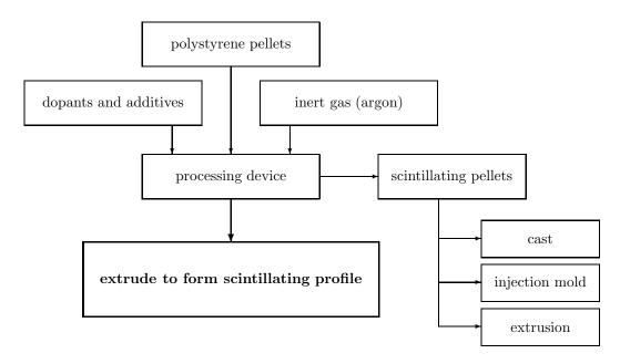
FIG. 5. Continuous in-line coloring and extrusion process (Method 2).
