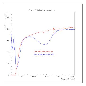
FIG. 2. Transmittance data of commercial polystyrene pellets.
