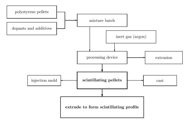
FIG. 4. Two-step process: batch coloring and extrusion (Method 1).
