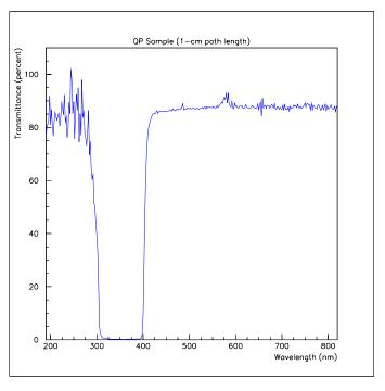
FIG. 3. Transmittance data of extruded plastic scintillator.
