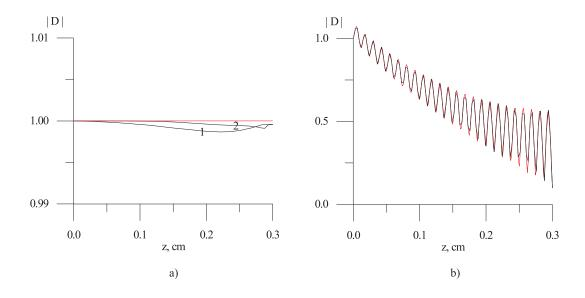
Figure 4: a) Reduced amplitudes of direct wave for L=0.3 cm,  $1-N_1=20, 2-N_1=50$  by scheme (3.12) with coefficients (2.8). b) Amplitudes of direct wave for L=0.3 cm,  $N_1=50$  (numerical and analytical solutions).
