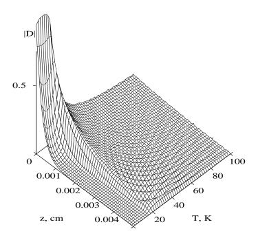
Figure 10: Evolution of diffracted wave amplitude under crystal heating to  $100~\mathrm{K}.$
