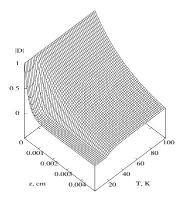
Figure 9: Evolution of direct wave amplitude under crystal heating to 100 K.
