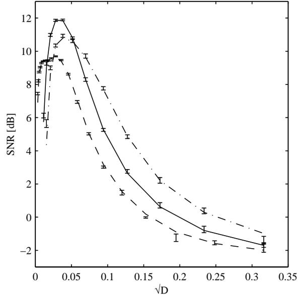
FIG. 8. Signal-to-noise ratio vs. noise amplitude for three different stimulus frequencies:  $\Omega = 0.1\pi$  (dashed),  $\Omega = 0.33\pi$  (solid) and  $\Omega = 0.5\pi$  (dash-dotted). Other parameters are  $\mu = 0.95$  and  $q = 0.05$ . Error bars show s.e.m. from simulated trains of 20,000 spikes.
