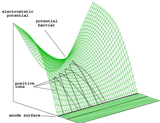
Figure 8: Potential distribution in front of the anode plane of HPD from Fig. 7. Positive ions of energy  $E_{ion}=44$  eV and emission angle normal to the anode surface start “climbing” the potential barrier ( $E_b=45$  eV) but eventually become repelled.
