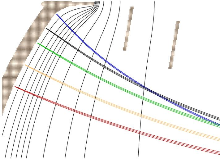
Figure 2: Incorrect electron focussing close to the periphery of the photocathode is due to the small radius of curvature of equipotential lines.
