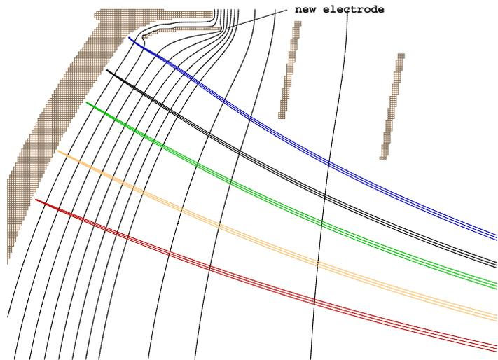
Figure 3: The new electrode allows the potential lines to be conducted out from the HPD through the created slot, curing the unwanted strong curvature of the equipotential lines seen in Fig. 3.
