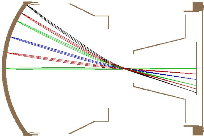
Figure 5: A cross-focussing 5-inch diameter HPD, with superior imaging characteristics. Electrodes are kept at the following potentials, from left to right, respectively: -20 kV, -19.97 kV, -19.4 kV, +100 V, and 0 V.
