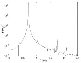
Figure 6: Power spectrum of the longitudinal wake potential for 30 bunches in the 5-cell  $\beta = 0.82$  cavity.
