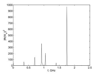
Figure 3: Power spectrum of the transverse wake potential for 30 bunches in the 5-cell  $\beta = 0.64$  cavity.
