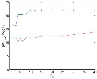
Figure 2: Maximum transverse wake potential for 5-cell APT SC cavities versus the number of bunches: circles for  $\beta = 0.64$ , stars for  $\beta = 0.82$ .
