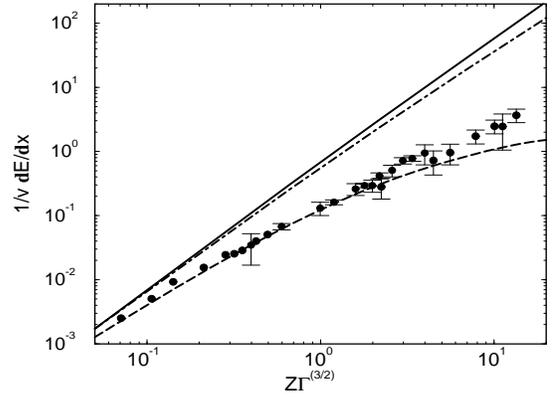
FIG. 7. The normalized friction coefficient (energy loss) for RPA (solid line), T-matrix result (dashed line) and Mermin DF result (dot-dashed line). The filled circles are simulation results [14] which reproduces experimental data [15,16].
