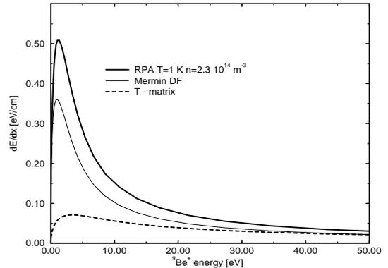
FIG. 4. The stopping power of  ${}^9\text{Be}^+$  ions in an electronic plasma versus ion energy. The classical Lindhard result (thick line) is compared with the Mermin result (thin line) and the T-matrix result (dashed line) of binary collisions (36). The plasma parameter is  $\Gamma = 1.65$ .
