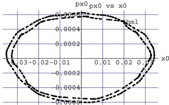
Figure 5.5: A plot showing the stability boundary for 500 turns for 2 dimensional motion in RHIC with the multipoles from  $k = 11$  to  $k = 20$  present. The multipoles for  $k = 2$  to  $k = 10$  have been corrected. The stability boundary in the high multipole limit is also shown. In the figure,  $px_0, x_0$  represent  $p_{x0}, x_0$ .
