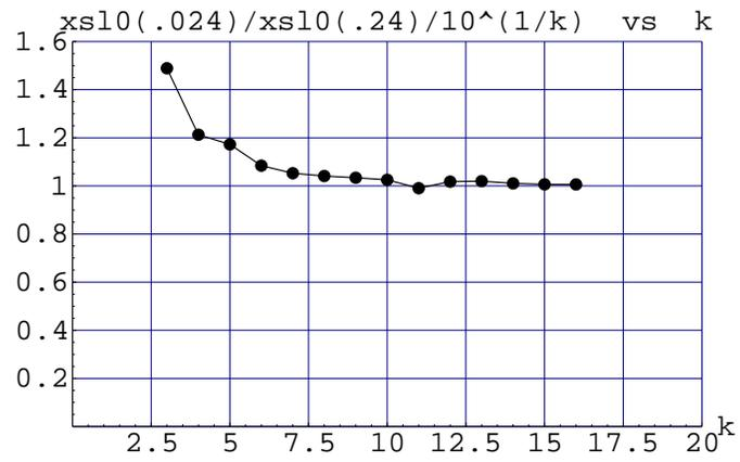
Figure 2.3: A plot showing that  $x_{sl0}$  depends on the multipole strength like  $x_{sl0} \sim b^{(1/k)}$  for large  $k$ , by comparing two cases where  $\mathbf{b}$  differs by a factor of 10. In the figure,  $x_{sl0}$  represents  $x_{sl0}$ .
