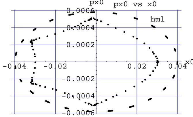
Figure 4.1: A plot of  $p_{x0}$  versus  $x_0$  showing the stability boundary for 2 dimensional motion in the simple one cell lattice with all multipoles from  $k = 2$  to  $k = 50$  at  $q_f$ . The stability boundary in the high multipole limit is also shown. In the figure,  $px0, x0$  represent  $p_{x0}, p_0$ .
