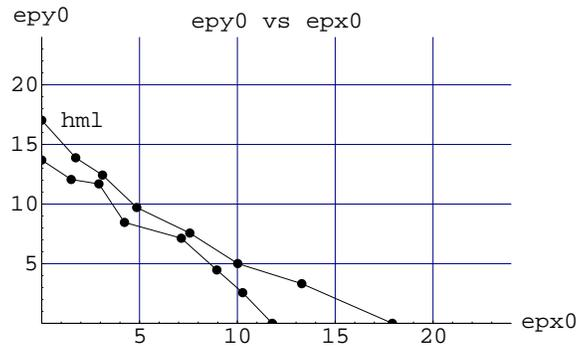
Figure 5.6: A plot showing the stability boundary for 500 turns for 4 dimensional motion for a RHIC lattice with all the multipoles from  $k = 2$  to  $k = 20$  present. The stability boundary in the high multipole limit is also shown. In the figure,  $\text{epy0}, \text{epX0}$  represent  $\epsilon_{y0}, \epsilon_{x0}$  are in mm-mrad.
