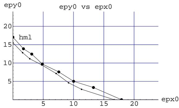
Figure 5.7: A plot showing the stability boundary for 500 turns for 4 dimensional motion for a RHIC lattice with the multipoles from  $k = 11$  to  $k = 20$  present. The multipoles for  $k = 2$  to  $k = 10$  have been corrected. The stability boundary in the high multipole limit is also shown. In the figure  $epy_0, epX_0$  represent  $\epsilon_{y0}, \epsilon_{x0}$  and are in mm-mrad.
