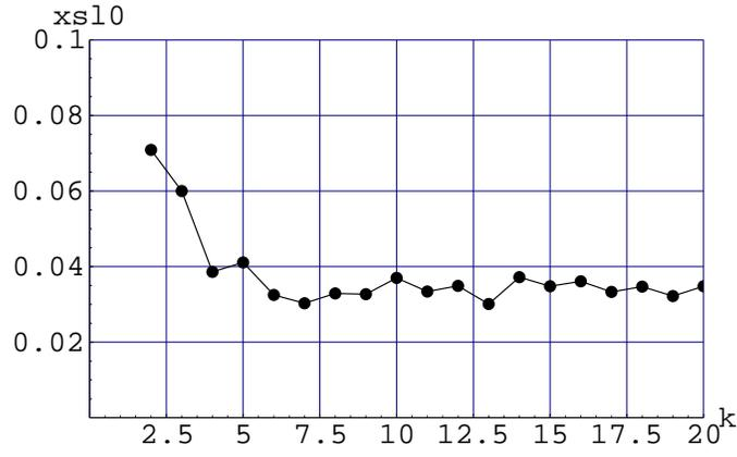
Figure 3.2: A plot of  $x_{sl0}$  versus  $k$  for the simple one cell lattice with a single multipole of order  $k$  at  $q_f$ , for 4 dimensional motion when  $p_{x0} = 0 = p_{y0}$  and  $\epsilon_{y0} = \epsilon_{x0}$ . In the figure, xsl0 represents  $x_{sl0}$  and is in meters.
