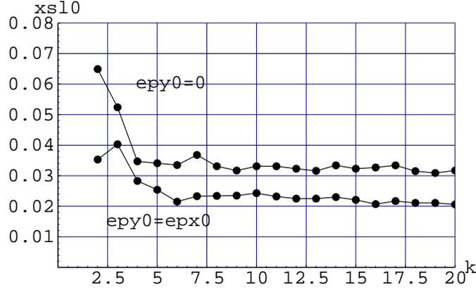
Figure 5.1: A plot of  $x_{sl0}$  versus  $k$  for RHIC. Each element has a single multipole of the same order,  $k$ . For one curve  $\epsilon_{y0} = 0$  and  $p_{x0} = p_{y0} = 0$ . For the other curve  $\epsilon_{y0} = \epsilon_{x0}$  and  $p_{x0} = p_{y0} = 0$ .  $x_{sl0}$  is computed for 500 turns. In the figure,  $xsl0, epy0, epx0$  represent  $x_{sl0}, \epsilon_{y0}, \epsilon_{x0}$ .
