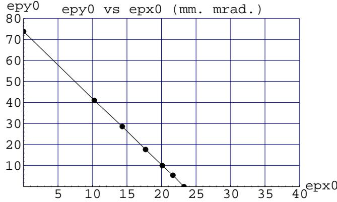
Figure 3.1: A plot showing the stability boundary in the hml for 4 dimensional motion, for the simple one cell lattice, as a plot of  $\epsilon_{y0}$  versus  $\epsilon_{x0}$ .  $\epsilon_{y0}$ ,  $\epsilon_{x0}$  represent  $\epsilon_{y0}$ ,  $\epsilon_{x0}$ .
