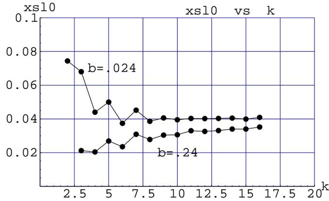
Figure 2.2: A plot showing how  $x_{sl0}$  versus  $k$  depends on the strength,  $\mathbf{b}$ , of the single multipole at  $q_f$  for the simple one cell lattice, by comparing two cases where  $\mathbf{b}$  differs by a factor of 10. In the figure  $x_{sl0}$  represents  $x_{sl0}$ .
