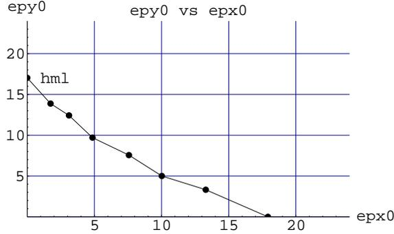
Figure 5.3: A plot showing the stability boundary in the high multipole limit for motion in 4 dimensional phase space for a RHIC lattice in  $\epsilon_{y0}$  vs  $\epsilon_{x0}$  space. Tracking runs of 500 turns were used with  $p_{x0} = p_{y0} = 0$  and with a single multipole with  $k = 20$  present in each element. In the figure,  $\text{epy0}, \text{epx0}$  represent  $\epsilon_{x0}, \epsilon_{x0}$  which are in mm mrad.
