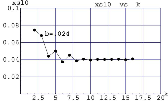
Figure 2.1: A plot of  $x_{s10}$  versus  $k$  for the simple one cell lattice with a single multipole of order  $k$  at  $q_f$ .  $x_{s10}$  is the largest  $x_0$  that is stable for 100 periods.  $p_{x0} = p_{y0} = y_0 = 0$  and 2 dimensional motion. In the figure xs10 represents  $x_{s10}$ .
