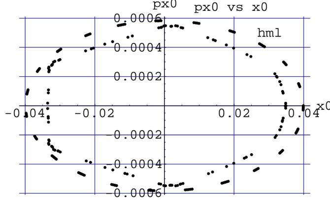
Figure 4.2: A plot of  $p_{x0}$  versus  $x_0$  showing the stability boundary for 2 dimensional motion in the simple one cell lattice with multipoles from  $k = 10$  to  $k = 50$  at  $q_f$ . The lower multipoles,  $k = 2$  to  $k = 9$  have been corrected. The stability boundary in the high multipole limit is also shown. In the figure,  $px0, x0$  represent  $p_{x0}, x_0$ .
