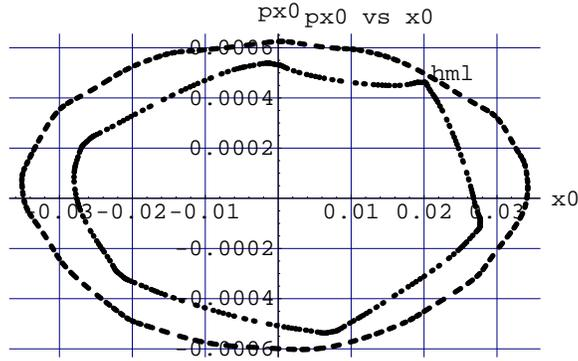
Figure 5.4: A plot showing the stability boundary for 500 turns for 2 dimensional motion in RHIC with all the multipoles from  $k = 2$  to  $k = 20$  present. The stability boundary in the high multipole limit is also shown. In the figure,  $px_0, x_0$  represent  $p_{x0}, x_0$ .
