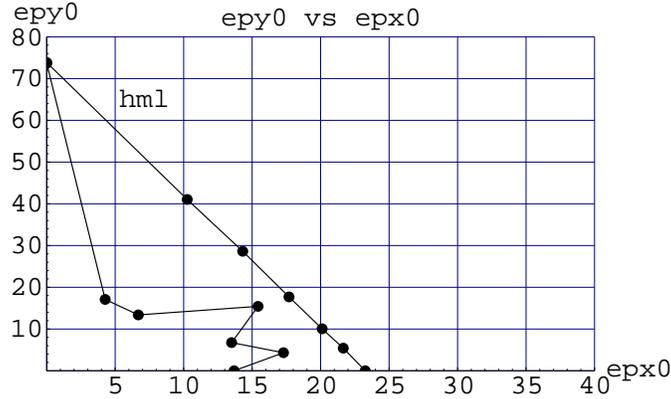
Figure 4.3: A plot of  $\epsilon_{y0}$  versus  $\epsilon_{x0}$  showing the stability boundary in  $\epsilon_{x0}$ ,  $\epsilon_{y0}$  space for 4 dimensional motion in the simple one cell lattice when all the multipoles from  $k = 2$  to  $k = 50$  are present at  $q_f$ . The stability boundary in the high multipole limit is also shown. In the figure, epy0,epx0 represent  $\epsilon_{y0}$ ,  $\epsilon_{x0}$ .
