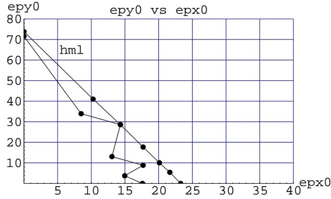
Figure 4.4: A plot of  $\epsilon_{y0}$  versus  $\epsilon_{x0}$  showing the stability boundary in  $\epsilon_{x0}, \epsilon_{y0}$  space for 4 dimensional motion in the simple one cell lattice when the multipoles from  $k = 10$  to  $k = 50$  are present at  $q_f$ . The multipoles from  $k = 2$  to  $k = 9$  have been corrected. The stability boundary in the high multipole limit is also shown. In the figure, epy0,epx0 represent  $\epsilon_{y0}, \epsilon_{x0}$ .
