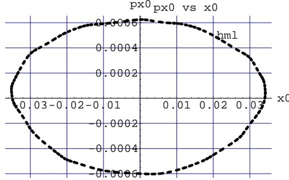
Figure 5.2: A plot showing the stability boundary for 500 turns in the high multipole limit for motion in 2 dimensional phase space for a RHIC lattice. In the figure,  $px_0, x_0$  represent  $p_{x0}, x_0$ .
