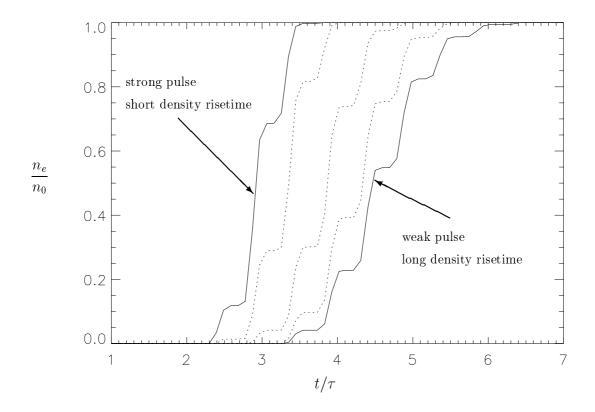
Figure 2. D. Bauer et al., "Generation of ultra-short ..."
