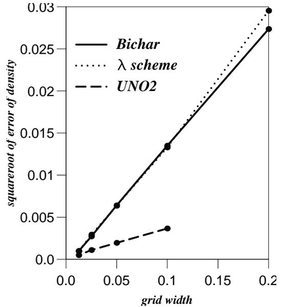
Figure 4: Comparison of convergence of the UNO-,  $\lambda$ - and bicharacteristic scheme
