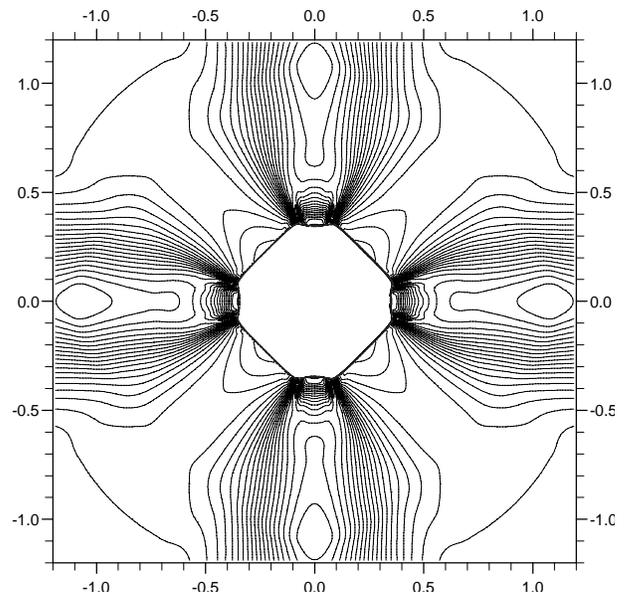
Figure 6: Isopycnic at  $t=0.2622$  (after fragmentation). The curvature of the Mach stem is below grid width and cannot be observed by shock capturing schemes in this resolution. Compare also fig. 7.
