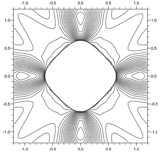
Figure 5: Isopycnic at  $t=0.1750$  (before fragmentation). The bold contour represents the leading shock wave.
