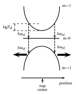
FIG. 1. Magnetic trapping of neutral atoms. We show the atomic potentials for the f = 1 trapping system, and how the radiofrequency field (frequency  $\omega_{\rm rf}$ ) can be used to control the trap depth  $k_BT_d$ . The resonant transition  $m = -1 \rightarrow m = 0 \rightarrow m = +1$  moves the atoms with kinetic energy larger than  $k_BT_d$  from the trapping state to a strongly nontrapping state.
