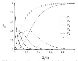
FIG. 3. The transition probabilities for the f = 2 multistate Landau-Zener model. The two-state solution is given by p, and goes clearly faster to unity with increasing  $\Omega_0^2/a$ than the corresponding five-state probability  $P_5$ .
