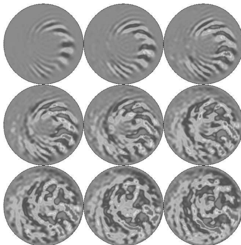
Figure 3: Time evolution of ion density in a simulation of tokamak plasma showing transition to a turbulent state. Time sequences advance from left to right, top row to bottom row.
