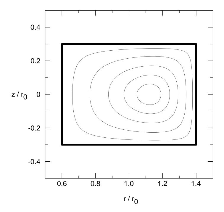
FIG. 1. Contours of constant  $\psi$  in the case that  $j_{\varphi} = \lambda r$ , for  $r_{-}/r_{0} = 0.6$ ,  $r_{+}/r_{0} = 1.4$  and  $L/r_{0} = 0.3$ . The ratio of magnetofluid pressure to poloidal magnetic field pressure  $(\beta_{p})$  in this case is about 1.1.
