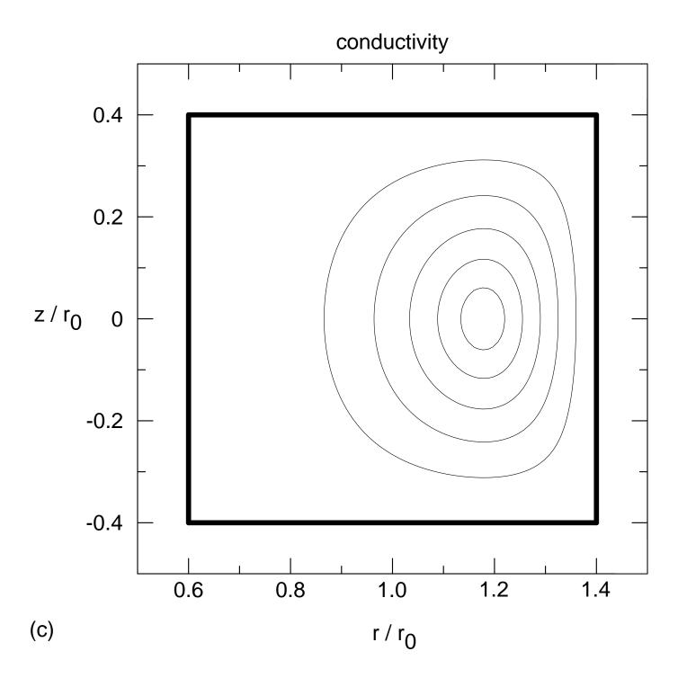
FIG. 2. (a) Contours of constant  $\psi$  (and pressure) in the case that  $j_{\varphi} = \lambda r \psi$ , for n = 0,  $\lambda r_0^4 = 29.375$ ,  $\delta/r_0 = 0.4$ , and  $L/r_0 = 0.4$ . (b) Current density contours, and (c) conductivity contours for the same set of parameters. The square box shows the location of the perfectly conducting, toroidal boundary. Note the non-coincidence of the conductivity contours and the magnetic surfaces. In this example,  $\beta_p \simeq 1.2$ .
