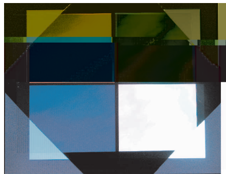
FIG. 5: Large-scale retardation uniformity of a transparency sheet in two dimensions. The transparency is placed between a 17" thin film transistor - liquid crystal display (TFT-LCD) computer monitor, source of polarized light with polarization at 45^\circ with respect to vertical, and a square polaroid film of similar size oriented to extinguish light in the absence of transparency. Transparency has its edges aligned with the screen. The color segments are generated in the computer by drawing filled rectangles in a drawing program. Three "pure" color quadrants provide information on uniformity at different wavelengths. In general it is expected that birefringence variation caused by non-uniformity of stretching should be similar for the three different colors, although somewhat smaller for red.
