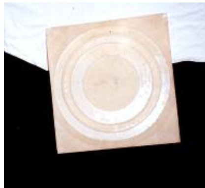
Fig.6: Fabricated 2-step Fresnel lens
