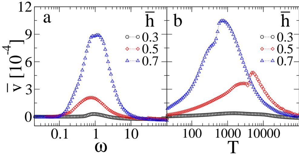
FIG. 4: Variation of the mean velocity  $\bar{v}$  in dependence of (a) the flashing ratio  $\omega$  (for  $T=500$ ) and (b) the flashing period  $T$  (for  $\omega = 1$ ) for various film thicknesses as given in the legends. The remaining parameters are as in Fig. 2.
