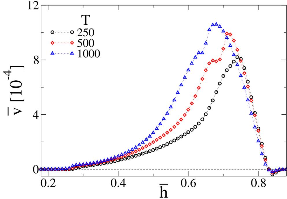
FIG. 3: Dependence of the mean velocity  $\bar{v}$  on the liquid level in the capacitor, i.e. on the mean film thickness  $\bar{h}$ , for various flashing periods  $T$  as indicated in the legend. The remaining parameters are as in Fig. 2.
