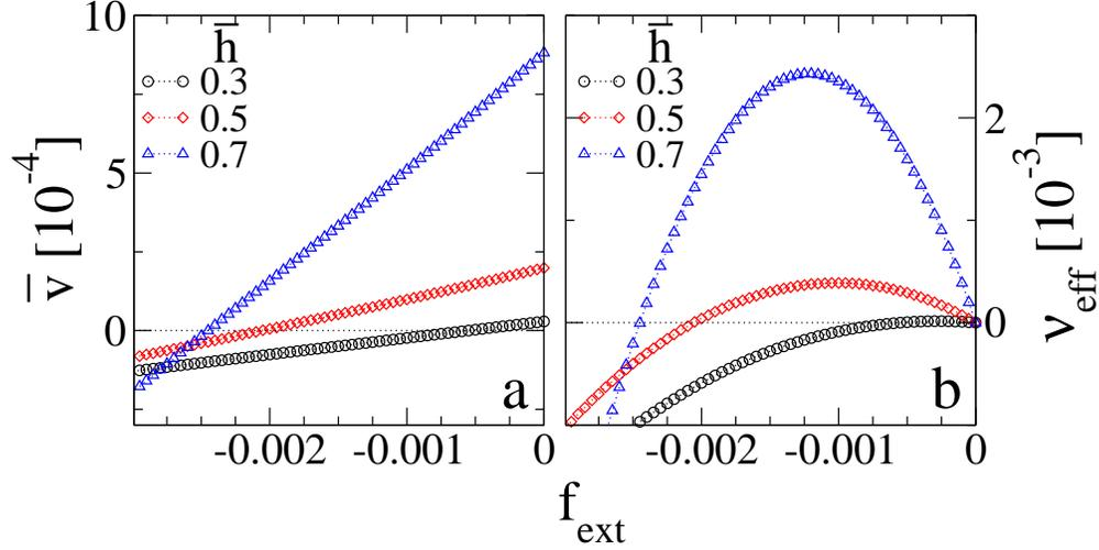
FIG. 5: The influence of an external load  $f_{\text{ext}}$ . Shown are the variations of (a) the mean velocity  $\bar{v}$  and (b) the transport efficiency  $\nu_{\text{eff}}$  with  $f_{\text{ext}}$  for various mean film thicknesses  $\bar{h}$  as indicated in the legends. The remaining parameters are as in Fig. 2 except for  $T = 500$ .
