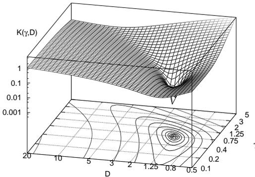
FIG. 2: Kullback distance between processes ( $\gamma_0 = 0.75$ ,  $D_0 = 1.25$ ) and  $(\gamma, D)$  as function of  $\gamma$  and  $D$  for  $\tau = 0.5$ . A distinct minimum at  $(\gamma, D) = (\gamma_0, D_0)$  is evident. The contour lines are located at  $z = 2^i$  for  $i = -11, \dots, 0$ . For the sake of clearness, the z-axis is scaled logarithmically.
