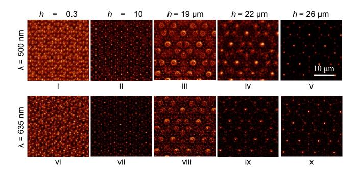
**Figure 2**. Field maps at different heights h above the quasi-crystal array of holes. The images were obtained by SNOM using illumination wavelengths of 500 nm (upper row) and 635 nm (lower row). Note the highly isolated hotspots observed at  $h=26~\mu m$  for the 500 nm excitation wavelength and at  $h=22~\mu m$  for the 635 nm excitation wavelength.
