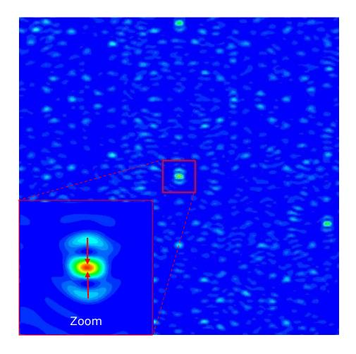
Figure 4. Theoretical calculations: subwavelength hot-spots formed at a height of  $12\mu m$  from the sample above the quasi-crystal array for a plane wave excitation at a wavelength of 635 nm.
