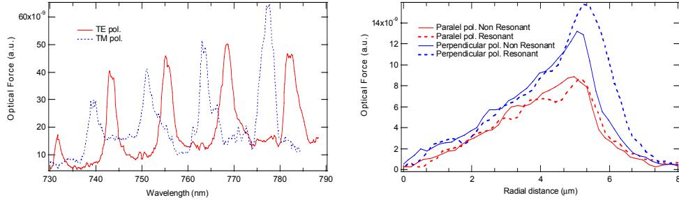
Fig. 3. Radial optical forces enhancement due to MDR for a 9  $\mu\text{m}$  sphere and polarizations as a function of: (left) wavelength; (right) radial distance.
