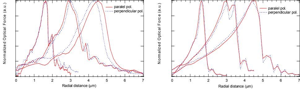
Fig. 2. Radial optical forces for 3, 6 and 9  $\mu\text{m}$  spheres: (left) experimental; (right) theory.
