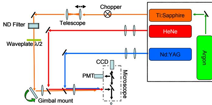
Fig. 1. Complete scheme for the double optical tweezers for ultra-sensitive force spectroscopy.
