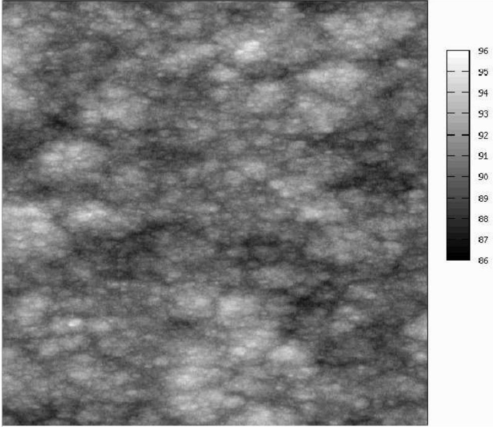
FIG. 3: Gray scale image of a morphology obtained by numerically solving the anisotropic KPZ equation. The image represents the central ( $512 \times 512$ ) part from the entire ( $1024 \times 1024$ ) simulated surface. The conditions at which the simulation is carried out are discussed in the text.
