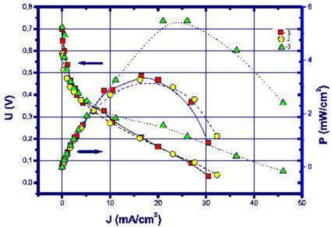
Figure 2: Plots of voltage  $U$  (left scale) and specific power (right scale) versus current density measured in a prototype FC. Curves 1–3 refer to three sequential experimental runs performed with a 10-min time interval.
