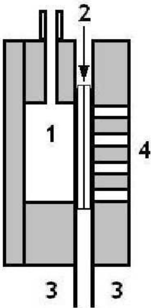
Figure 1: Schematic diagram of the electrochemical cell involving a cathode half-MEA: (1) liquid fuel container; (2) membrane-electrode assembly (see the text for details); (3) plate electrodes with holes; (4) case with air channels. Spacers and screws are not shown.
