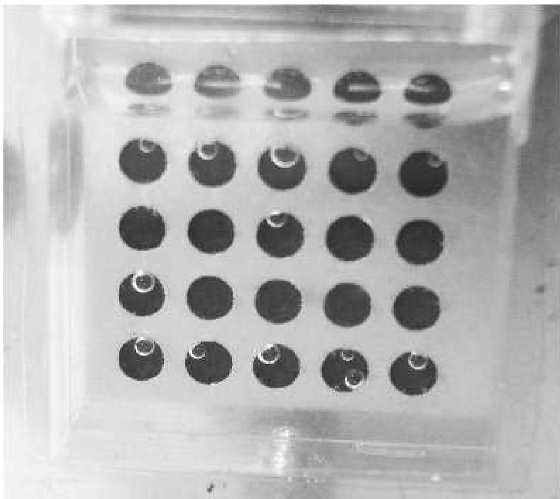
Figure 3:  $CO_2$  evolution on the anode of operating FC.
