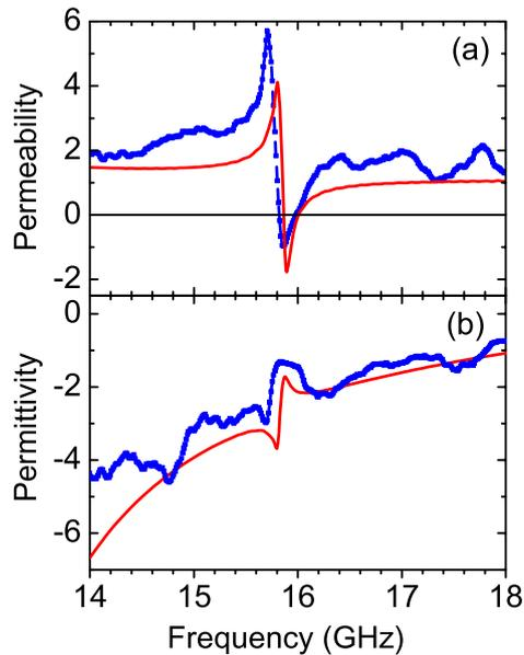
Figure 4 Extracted permittivity  $\epsilon$  (a) and permeability  $\mu$  (b) of a periodic array of wire-pair unit cells, using the simulated (red solid curves) and measured (blue dotted curves) transmission and reflection data.
