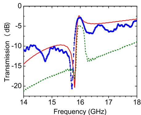
Figure 2. Simulated (red solid curve) and measured (blue dotted curve) transmission spectra for electromagnetic radiation incident on the wire-pair structures. The green dashed curve shows the simulated transmission spectrum for a 5-layer sample.
