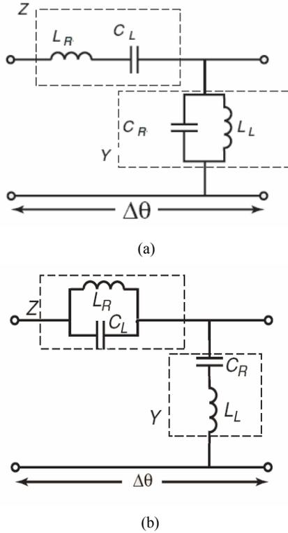
**Fig. 1** The lumped LC unit cell for (a) a CRLH phase-shifting line and (b) a dual CRLH phase-shifting line.
