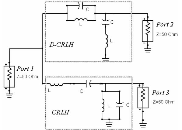
Fig. 4 Equivalent circuit of a dual band balun.
