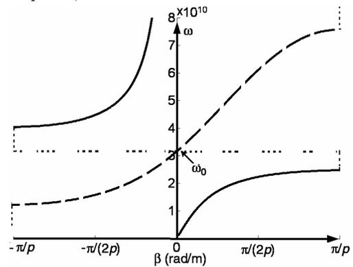
**Fig. 2** Dispersion diagram for the balanced case of a D-CRLH line (solid line) or a standard CRLH line (dashed)
