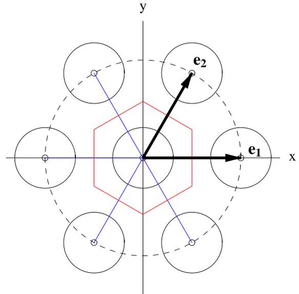
FIG. 1. The Wigner-Seitz cell (red) with the central inclusion (coated cylinder with  $r_c = 0.03d$ ,  $r_s = 0.31d$  and  $d = 1$ ) and the nearest neighbours (located along the dashed circle) for a hexagonal array. The centers of the nearest neighbours are given by the lattice vectors  $\mathbf{R}_p$  for  $p \in \{(-1, 0), (-1, 1), (0, -1), (0, 1), (1, -1), (1, 0)\}$ . We also show the fundamental translation vectors  $\mathbf{e}_1 = d(1, 0)$  and  $\mathbf{e}_2 = d(1/2, \sqrt{3}/2)$ .
