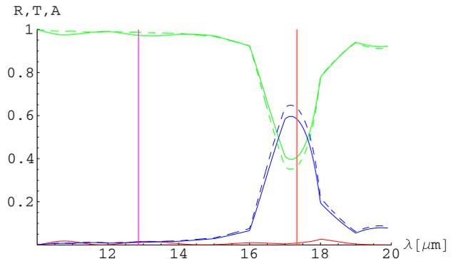
FIG. 7. TM polarization: Reflectance (red), transmittance (green) and absorptance (blue) for a stack of solid cylinders of refractive index  $n_c = n_{\text{Al}_2\text{O}_3}$  and radius  $r_c$  (dashed curves), and for a stack of coated cylinders (solid curves). In both cases the stack consists of 30 gratings of cylinders, and represents a “slice” from a 2-dimensional hexagonal array. The vertical magenta lines mark the two solutions  $\lambda_1$  and  $\lambda_2$ , of (57).
