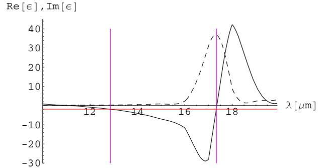
FIG. 3. Real (solid curve) and imaginary (dashed curve) part of  $\text{Al}_2\text{O}_3$  relative dielectric constant versus wavelength. The horizontal red line shows  $-n_d^2$ , while the vertical magenta lines mark the two solutions  $\lambda_1$  and  $\lambda_2$ , of (57).
