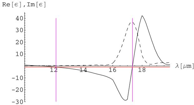
FIG. 4. Real (solid curve) and imaginary (dashed curve) part of  $\text{Al}_2\text{O}_3$  relative dielectric constant versus wavelength. The horizontal red line shows  $-n_m^2 = -1$ , while the vertical magenta lines mark the two solutions  $\tilde{\lambda}_1, \tilde{\lambda}_2$ , of (62).
