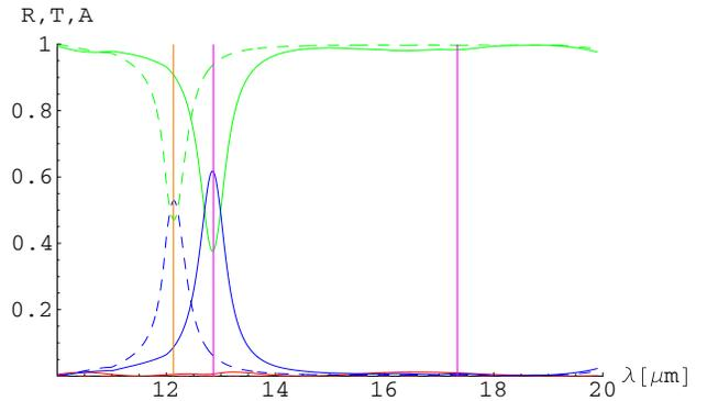
FIG. 5. TE polarization: Reflectance (red), transmittance (green) and absorbance (blue) for a stack of solid cylinders of refractive index  $n_c = n_{\text{Al}_2\text{O}_3}$  and radius  $r_c = 0.03\mu\text{m}$  (dashed curves), and for a stack of coated cylinders (solid curves). In both cases the stack consists of 30 gratings of cylinders, and represents a “slice” from a 2-dimensional hexagonal array. The vertical magenta lines mark the two solutions  $\lambda_1$  and  $\lambda_2$ , of (57).
