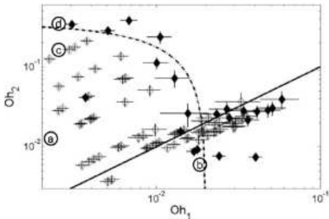
FIG. 5: Phase plane  $Oh_1 - Oh_2$  ( $Bo < 0.1$ ). Experimental results: Total coalescence ( $\blacklozenge$ ) vs. partial coalescence ( $\diamond$ ). The dashed line corresponds to the linear relationship (11). The solid line corresponds to the equality of both Ohnesorge numbers. Circled letters indicate the position of the four snapshots (Fig. 2).
