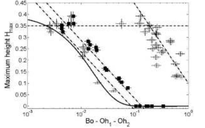
FIG. 11: Maximum droplet elevation vs. Ohnesorge 1 ( $\Delta$ ), Ohnesorge 2 ( $\blacksquare$ ), and Bond ( $\circ$ ). Dashed lines are guides for the eyes. The solid line corresponds to the forecast of the linear waves theory (Eq. (26)).
