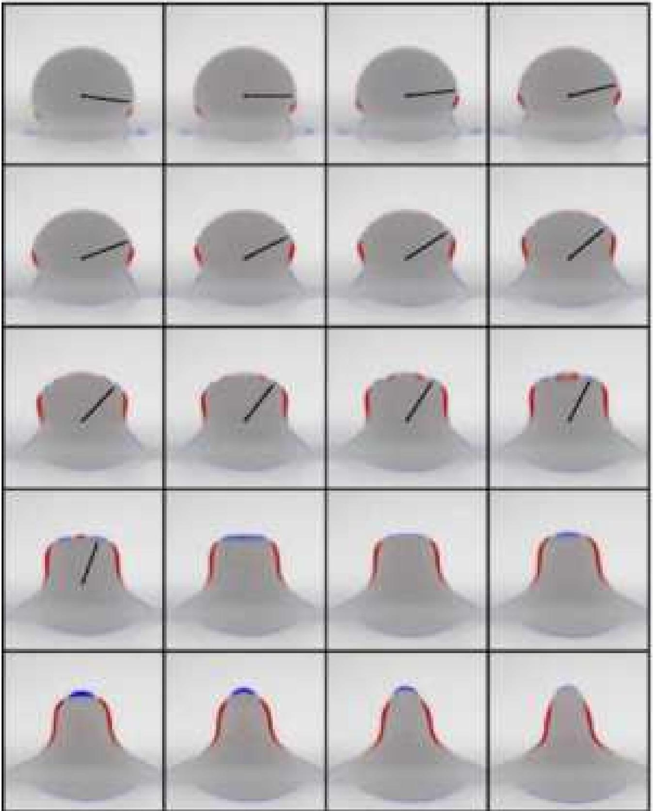
FIG. 8: (Color online) Capillary wave propagation obtained by image subtraction. The blue interface is progressing toward fluid 2, while the red interface is receding. The time step is equal to  $0.045\tau_\sigma$ .  $Bo = 0.15$ ,  $Oh_1 = 0.002$ ,  $Oh_2 = 0.014$
