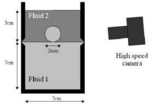
FIG. 1: Experimental setup: A container is filled with two immiscible fluids. A droplet of fluid 1 is falling through fluid 2, before coalescing with the fluid 1 bulk phase. The same experiment can be conducted when fluid 1 is lighter than fluid 2 (the droplet is going up).
