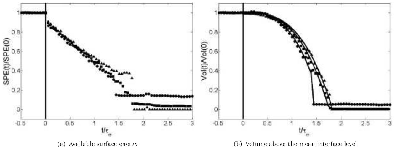
FIG. 7: Evolution of the global quantities for a self-similar partial coalescence ( $\bullet$  -  $Oh_2 \ll Oh_{2c}$ ), an attenuated partial coalescence ( $\blacksquare$  -  $Oh_2 \lesssim Oh_{2c}$ ), and a total coalescence ( $\blacktriangle$  -  $Oh_2 > Oh_{2c}$ ).
