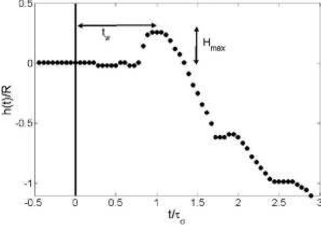
FIG. 9: Evolution of the height of the droplet  $h$  for a self-similar partial coalescence ( $\bullet$  -  $Oh_2 \ll Oh_{2c}$ ), an attenuated partial coalescence ( $\blacksquare$  -  $Oh_2 \lesssim Oh_{2c}$ ), and a total coalescence ( $\blacktriangle$  -  $Oh_2 > Oh_{2c}$ ).
