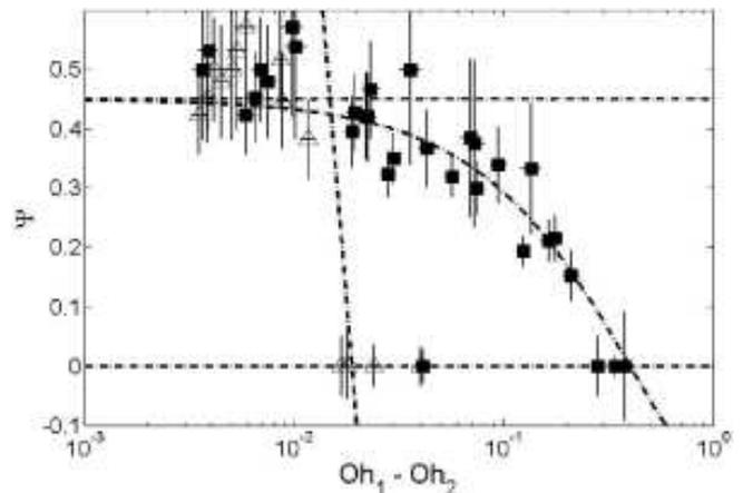
FIG. 4: Ohnesorge 1 ( $\Delta$ ) and Ohnesorge 2 ( $\blacksquare$ ) influences on the radius ratio  $\Psi$ . The Bond number is smaller than 0.1, and the other Ohnesorge number is smaller than  $7.5 \times 10^{-3}$ . Dashed lines are guides for the eyes.
